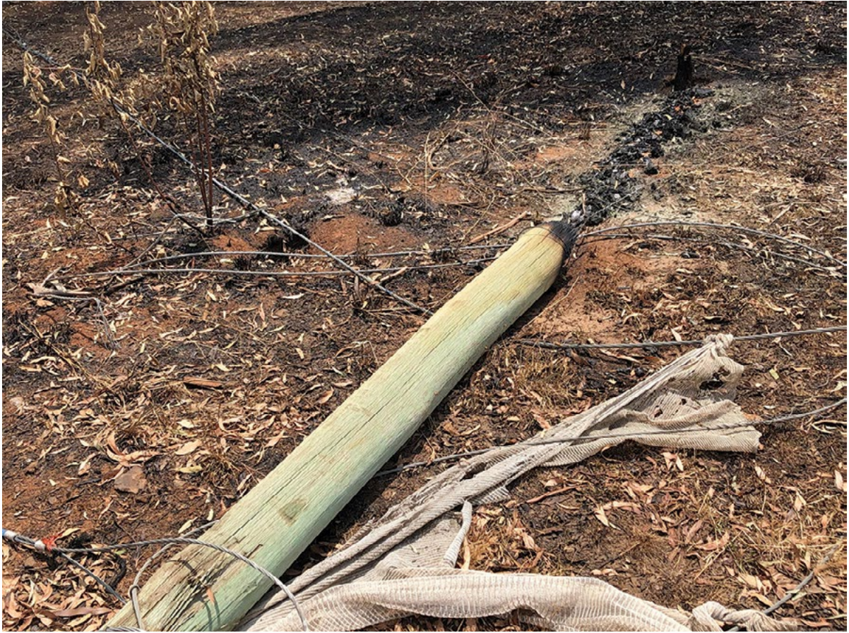
Figure 18. Chemical ash residues from burnt treated pine poles present a risk to stock and human health and require careful management.
