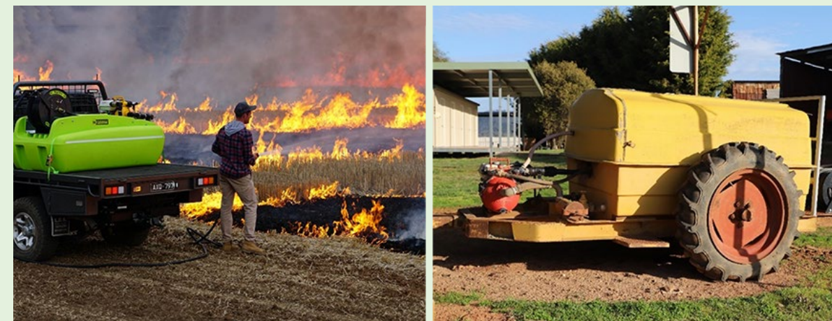
Figure 49. Firefighting units can be purpose made (left, photo: Trans Tank, https://www.tti.com.au/product/firedefence-portable-fire-fighter-800-litres/ ) or retrofitted to old orchard sprayer vats (right).
