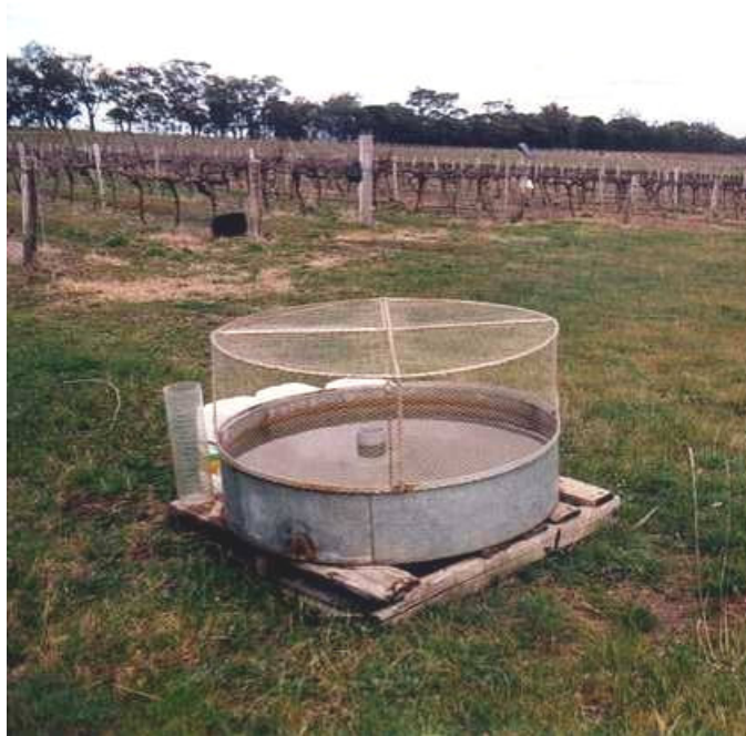
Photo 3: Class A Pan – measures evaporation
